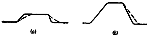
FIG. 6-7.—Response to (a) weak signals and (b) overloading signals for feedback pair (solid line), and narrowband two-stage amplifier with same gain distribution between stages as feedback pair (dashed line).
