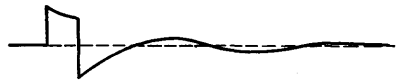
FIG. 3-6.—Waveform of pulse obtained from several successive coupling-circuit stages. There is one crossing of the baseline for each coupling circuit.
